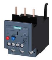
Overload relay 47...57 A Thermal For motor protection Size S2, Class 10 Contactor mounting Main circuit: Screw Auxiliary circuit: Screw Manual-Automatic-Reset
