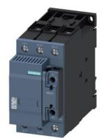
capacitor contactor, AC-6b 75 kVAr, / 400 V, 3-pole, 230 V AC, 50 Hz, auxiliary contacts: 1 NO + 1 NC, screw terminal
