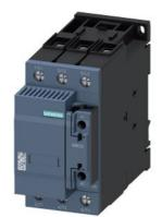
capacitor contactor, AC-6b 50 kVAr, / 400 V, 3-pole, 230 V AC, 50 Hz, auxiliary contacts: 1 NO + 1 NC, screw terminal
