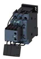
capacitor contactor, AC-6b 16.7 kVAr, / 400 V, 3-pole, 230 V AC, 50 Hz, auxiliary contacts: 1 NO + 2 NC, screw terminal
