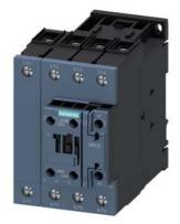
contactor AC-1, 110 A, 400 V / 40 °C, 4-pole, 220 V AC, 50 Hz / 240 V, 60 Hz, auxiliary contacts: 1 NO + 1 NC, screw terminal
