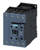
contactor AC-1, 60 A, 400 V / 40 °C, 4-pole, 175-280 V AC/DC, 50/60 Hz, with integrated varistor, auxiliary contacts: 1 NO + 1 NC, screw terminal, size: S2
