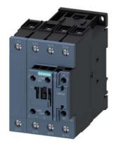
contactor AC-1, 60 A, 400 V / 40 °C, 4-pole, 220 V AC, 50 Hz / 240 V, 60 Hz, auxiliary contacts: 1 NO + 1 NC, screw terminal, size: S2
