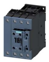
contactor AC-1, 60 A, 400 V / 40 °C, 4-pole, 110 V AC, 50 Hz, auxiliary contacts: 1 NO + 1 NC, screw terminal
