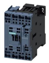
contactor AC-1, 35 A, 400 V / 40 °C, 4-pole, 110 V DC, auxiliary contacts: 1 NO + 1 NC, spring-loaded terminal, size: S0
