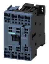
contactor AC-1, 35 A, 400 V / 40 °C, 4-pole, 24 V DC, auxiliary contacts: 1 NO + 1 NC, spring-loaded terminal
