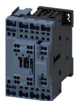
contactor AC-1, 35 A, 400 V / 40 °C, 4-pole, 230 V AC, 50 Hz, auxiliary contacts: 1 NO + 1 NC, spring-loaded terminal
