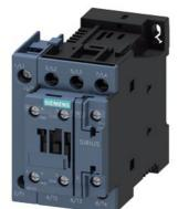
contactor AC-1, 35 A, 400 V / 40  $^\circ\text{C},$  4-pole, 48 V DC, auxiliary contacts: 1 NO + 1 NC, screw terminal
