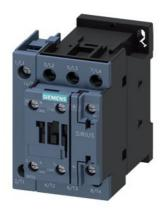
contactor AC-1, 35 A, 400 V / 40 °C, 4-pole, 230 V AC, 50 Hz, auxiliary contacts: 1 NO + 1 NC, screw terminal
