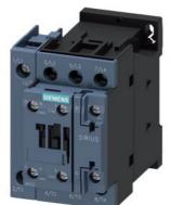
contactor AC-1, 35 A, 400 V / 40  $^\circ\text{C},$  4-pole, 24 V AC, 50 Hz, auxiliary contacts: 1 NO + 1 NC, screw terminal
