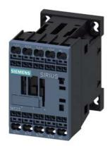
contactor AC-1, 22 A, 400 V / 40  $^{\circ}\text{C},$  4-pole, 208 V AC, 50/60 Hz, spring-loaded terminal
