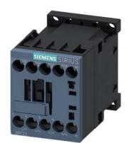
contactor AC-1, 18 A, 400 V / 40  $^\circ\text{C},$  4-pole, 24 V AC, 50/60 Hz, screw terminal
