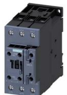
power contactor, AC-3e/AC-3, 80 A, 37 kW / 400 V, 3-pole, 230 V AC, 50 Hz, auxiliary contacts: 1 NO + 1 NC, screw terminal
