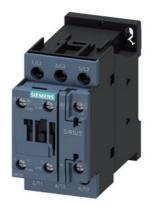
Power contactor, AC-3 32 A, 15 kW / 400 V 1 NO + 1 NC, 220 V AC, 50 Hz 240 V, 60Hz, 3-pole, Size S0, screw terminals
