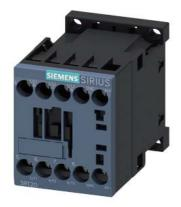
power contactor, AC-3e/AC-3, 16 A, 7.5 kW / 400 V, 3-pole, 60 V DC, auxiliary contacts: 1 NC, screw terminal, size: S00  $\,$
