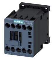
power contactor, AC-3e/AC-3, 16 A, 7.5 kW / 400 V, 3-pole, 60 V DC, auxiliary contacts: 1 NO, screw terminal, size: S00  $\,$
