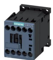
power contactor, AC-3e/AC-3, 16 A, 7.5 kW / 400 V, 3-pole, 400 V AC, 50 Hz / 400-440 V, 60 Hz, auxiliary contacts: 1 NC, screw terminal, size: S00
