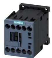
contactor, NEMA version, 5 HP, 460 / 575 V, 3-pole, 24 V AC, 50/60 Hz, auxiliary contacts: 1 NO, screw terminal, size: S00
