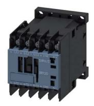
power contactor, AC-3e/AC-3, 12 A, 5.5 kW / 400 V, 3-pole, 24 V DC, 0.7-1.25\* Us, with integrated varistor, auxiliary contacts: 1 NC, ring cable lug connection, size: S00
