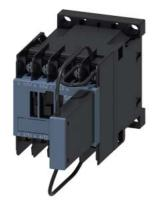
traction contactor, AC-3e/AC-3, 12 A, 5.5 kW / 400 V, 3-pole, 24 V DC, 0.7-1.25  $^{\star}$  Us, with integrated suppressor diode, auxiliary contacts: 1 NC, ring cable lug connection, size: S00, with plugged on series resistor
