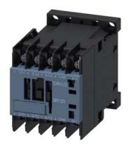
power contactor, AC-3e/AC-3, 12 A, 5.5 kW / 400 V, 3-pole, 24 V DC, 0.7-1.25 $^{\star}$  Us, with integrated suppressor diode, auxiliary contacts: 1 NC, ring cable lug connection, size: S00, suitable for PLC outputs, not expandable with auxiliary switch
