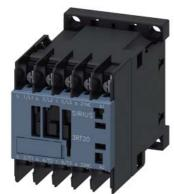
power contactor, AC-3e/AC-3, 12 A, 5.5 kW / 400 V, 3-pole, 200 V AC, 50 Hz / 200-220 V, 60 Hz, auxiliary contacts: 1 NC, ring cable lug connection, size: S00
