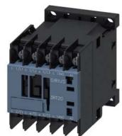
power contactor, AC-3e/AC-3, 12 A, 5.5 kW / 400 V, 3-pole, 200 V AC, 50 Hz / 200-220 V, 60 Hz, auxiliary contacts: 1 NO, ring cable lug connection, size: S00
