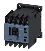
power contactor, AC-3e/AC-3, 12 A, 5.5 kW / 400 V, 3-pole, 100 V AC, 50 Hz / 100-110 V, 60 Hz, auxiliary contacts: 1 NC, ring cable lug connection, size: S00
