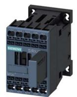
power contactor, AC-3e/AC-3, 12 A, 5.5 kW / 400 V, 3-pole, 24 V DC, 0.85-1.85\* Us, with varistor plugged on, auxiliary contacts: 1 NC, spring-loaded terminal, size: S00, not expandable with auxiliary switch
