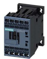
power contactor, AC-3e/AC-3, 12 A, 5.5 kW / 400 V, 3-pole, 24 V DC, 0.85-1.85\* Us, with integrated diode, auxiliary contacts: 1 NC, spring-loaded terminal, size: S00, not expandable with auxiliary switch
