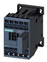
power contactor, AC-3e/AC-3, 12 A, 5.5 kW / 400 V, 3-pole, 24 V DC, 0.7-1.25\* Us, with varistor plugged on, auxiliary contacts: 1 NO, spring-loaded terminal, size: S00, not expandable with auxiliary switch
