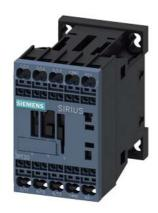
power contactor, AC-3e/AC-3, 12 A, 5.5 kW / 400 V, 3-pole, 24 V DC, 0.85-1.85  $^{\star}$  Us, auxiliary contacts: 1 NO, spring-loaded terminal, size: S00, not expandable with auxiliary switch
