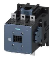
power contactor, AC-3e/AC-3 500 A, 250 kW / 400 V AC (50-60 Hz) / DC Uc: 380-420 V 3-pole, auxiliary contacts 2 NO + 2 NC drive: conventional main circuit: busbar control and auxiliary circuit: screw terminal
