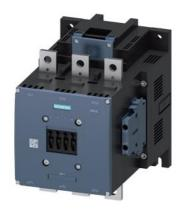
power contactor, AC-3e/AC-3 500 A, 250 kW / 400 V AC (50-60 Hz) / DC Uc: 240-277 V 3-pole, auxiliary contacts 2 NO + 2 NC drive: conventional main circuit: busbar control and auxiliary circuit: screw terminal
