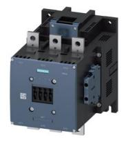
power contactor, AC-3e/AC-3 500 A, 250 kW / 400 V AC (50-60 Hz) / DC Uc: 575-600 V 3-pole, auxiliary contacts 2 NO + 2 NC drive: conventional main circuit: busbar control and auxiliary circuit: screw terminal
