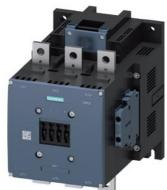
power contactor, AC-3e/AC-3 500 A, 250 kW / 400 V AC (50-60 Hz) / DC Uc: 500-550 V 3-pole, auxiliary contacts 2 NO + 2 NC drive: conventional main circuit: busbar control and auxiliary circuit: screw terminal
