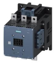
power contactor, AC-3e/AC-3 500 A, 250 kW / 400 V AC (50-60 Hz) / DC Uc: 440-480 V 3-pole, auxiliary contacts 2 NO + 2 NC drive: conventional main circuit: busbar control and auxiliary circuit: spring-loaded terminal
