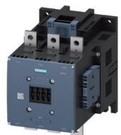
power contactor, AC-3e/AC-3 500 A, 250 kW / 400 V AC (50-60 Hz) / DC Uc: 110-127 V 3-pole, auxiliary contacts 2 NO + 2 NC drive: conventional main circuit: busbar control and auxiliary circuit: spring-loaded terminal
