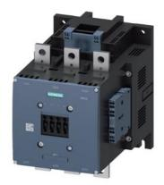
power contactor, AC-3e/AC-3 500 A, 250 kW / 400 V AC (50-60 Hz) / DC Uc: 23-26 V 3-pole, auxiliary contacts 2 NO + 2 NC drive: conventional main circuit: busbar control and auxiliary circuit: spring-loaded terminal
