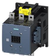
power contactor, AC-3e/AC-3 400 A, 200 kW / 400 V AC (50-60 Hz) / DC 96-127 V x (0.8-1.1) F-PLC input 24 V DC 3-pole, auxiliary contacts 2 NO + 2 NC drive: electronic main circuit: busbar control and auxiliary circuit: screw terminal
