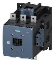
power contactor, AC-3e/AC-3 400 A, 200 kW / 400 V AC (50-60 Hz) / DC Uc: 200-277 V PLC input 24 V DC 3-pole, auxiliary contacts 2 NO + 2 NC drive: electronic main circuit: busbar control and auxiliary circuit: screw terminal
