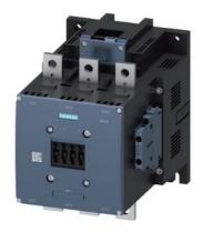
power contactor, AC-3e/AC-3 400 A, 200 kW / 400 V AC (50-60 Hz) / DC Uc: 96-127 V PLC input 24 V DC 3-pole, auxiliary contacts 2 NO + 2 NC drive: electronic main circuit: busbar control and auxiliary circuit: screw terminal
