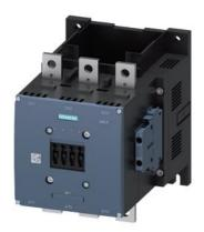
power contactor, AC-3e/AC-3 400 A, 200 kW / 400 V without operating mechanism 3-pole, auxiliary contacts 2 NO + 2 NC main circuit: busbar control and auxiliary circuit: screw terminal
