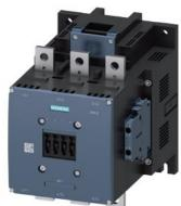
power contactor, AC-3e/AC-3 400 A, 200 kW / 400 V AC (50-60 Hz) / DC Uc: 200-220 V 3-pole, auxiliary contacts 2 NO + 2 NC drive: conventional main circuit: busbar control and auxiliary circuit: screw terminal
