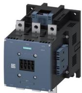
power contactor, AC-3e/AC-3 400 A, 200 kW / 400 V AC (50-60 Hz) / DC Uc: 200-277 V PLC input 24 V DC 3-pole, auxiliary contacts 2 NO + 2 NC drive: electronic main circuit: busbar control and auxiliary circuit: spring-loaded terminal
