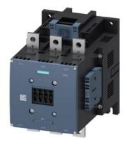
power contactor, AC-3e/AC-3 400 A, 200 kW / 400 V AC (50-60 Hz) / DC Uc: 110-127 V 3-pole, auxiliary contacts 2 NO + 2 NC drive: conventional main circuit: busbar control and auxiliary circuit: spring-loaded terminal
