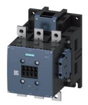
power contactor, AC-3e/AC-3 300 A, 160 kW / 400 V, AC (50-60 Hz) / DC Uc: 380-420 V 3-pole, auxiliary contacts 2 NO + 2 NC drive: conventional main circuit: busbar control and auxiliary circuit: screw terminal
