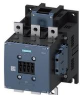
power contactor, AC-3e/AC-3 300 A, 160 kW / 400 V, AC (50-60 Hz) / DC Uc: 240-277 V 3-pole, auxiliary contacts 2 NO + 2 NC drive: conventional main circuit: busbar control and auxiliary circuit: screw terminal
