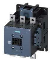
power contactor, AC-3e/AC-3 300 A, 160 kW / 400 V, AC (50-60 Hz) / DC Uc: 575-600 V 3-pole, auxiliary contacts 2 NO + 2 NC drive: conventional main circuit: busbar control and auxiliary circuit: screw terminal
