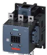
power contactor, AC-3e/AC-3 300 A, 160 kW / 400 V, AC (50-60 Hz) / DC Uc: 110-127 V 3-pole, auxiliary contacts 2 NO + 2 NC permanently mounted drive: conventional main circuit: busbar control and auxiliary circuit: screw terminal
